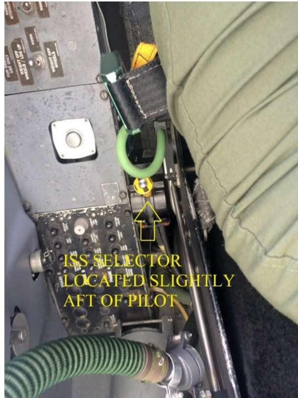
Figure 14: Location of ISS Mode Selector.
