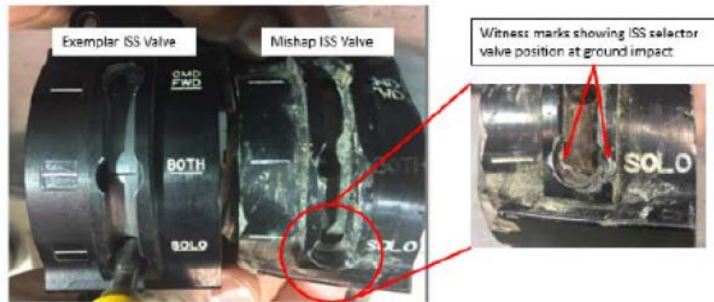
Figure 9: Exemplar and Mishap ISS Valve with Witness Marks (Tab H-18)
