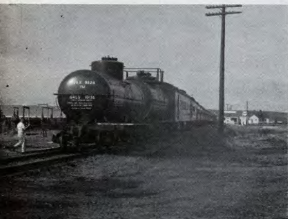
Above, the Missile Test Train waits on a siding at Bitter Creek, Wyo. The two tank cars are to transport fuel and water. Boeing representative at the left is taking grade measurements.
