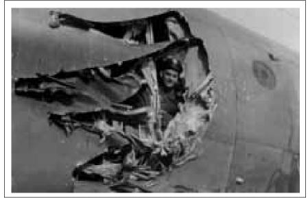
Pilot B.J. Anderson peers through the rip in his C-54's fuselage. He was taking off from Celle, Germany, when the hydraulic line to the C-54's No. 2 engine ruptured. Despite attempts to shut it down, the engine continued to accelerate and the propeller then sheared off and cut into the side of the fuselage. Anderson and his crew made a safe landing back at Celle.
