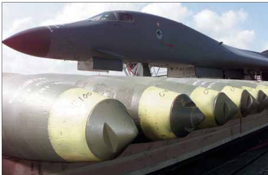
Today, B-1Bs carry dumb bombs like these Mk 82s. Soon, all bombers will have capability for precision weapons and USAF will be able to merge mass and precision in the same platforms.
