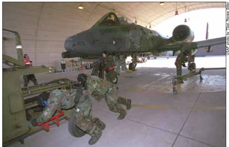
A-10 munitions load crew members from the 25th Fighter Squadron, Osan AB, South Korea, clear the ammunition-loading adaptor while the crew chief fuels the aircraft during a combat employment readiness exercise in January.
