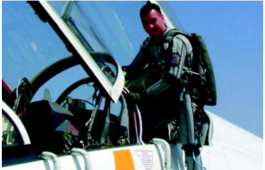
At the USAF Test Pilot School, Edwards AFB, Calif., Capt. Aaron George climbs out of a T-38 after testing a Swiss-made, liquid-filled, full-body anti-gravity suit. The new aircrew protection concept uses hydrostatic force to regulate suit pressure—a possible improvement over current compressed-air anti-g suits.
