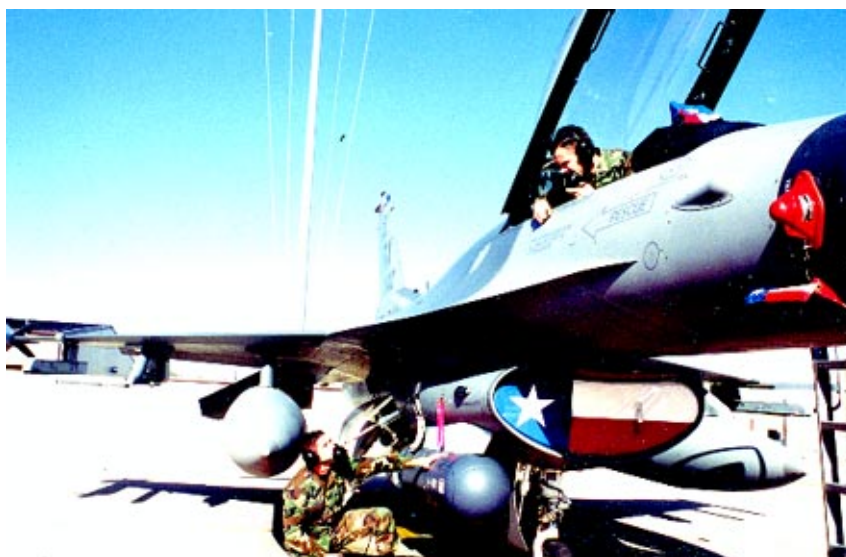
SSgts. Ryan Jones (left) and Charles Yaws ensure proper placement of a Litening II targeting pod on an F-16 from the 301st Fighter Wing (AFRC). The precision attack targeting system allows F-16 pilots to identify targets at long range, night or day, and drop extremely accurate laser-guided weapons.
