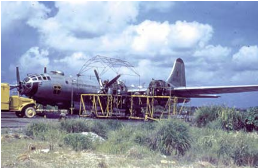
World War II-era B-29s were a mainstay of the interdiction effort on the peninsula. The coming of the MiG-15s, however, posed a lethal threat, and USAF soon retired the Superfortress. Here, a B-29 gets an engine change.
