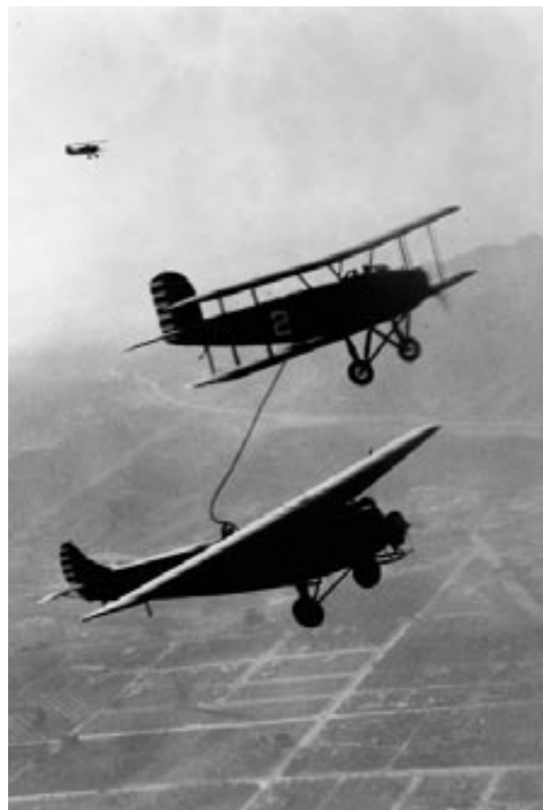
Eaker was involved with many prominent airpower events, including the flight of Question Mark, shown here. In 1929, Question Mark demonstrated aerial refueling possibilities and stayed aloft for almost seven days. Here, Question Mark takes on fuel from a tanker flying above it.
