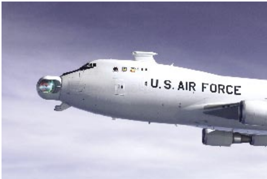
Here is the business end of the Airborne Laser. While electric lasers are developing apace, their power doesn’t compare with chemical lasers like that on the ABL. Directed energy holds huge promise for fast engagement of targets.
