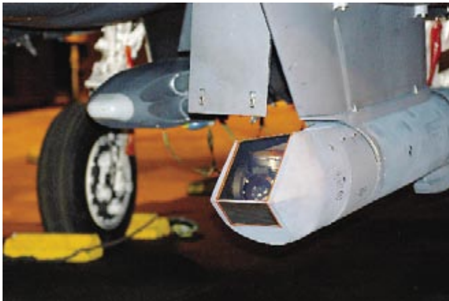
Pictured are Sniper Advanced Targeting Pods on F-15Es from RAF Lakenheath, UK. Intended to offer greater precision in aiming laser guided bombs, the pods have provided bonus surveillance and bomb damage assessment functions now widely employed in Southwest Asia. The Sniper can "talk" directly to controllers on the ground.
