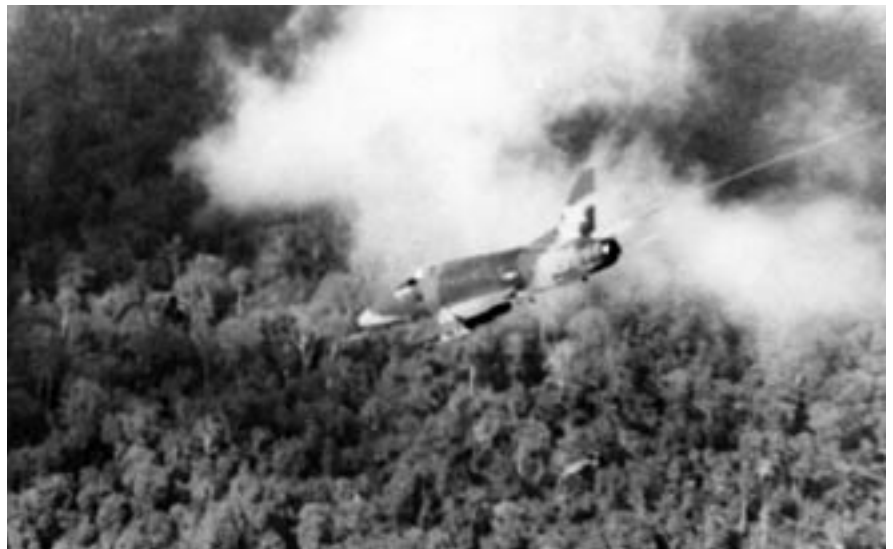
In Vietnam, new radar systems allowed fighters without ground target acquisition radars, such as this F-100, to accurately provide air support. Sky Spot would track the attack aircraft's position relative to a desired release point.
