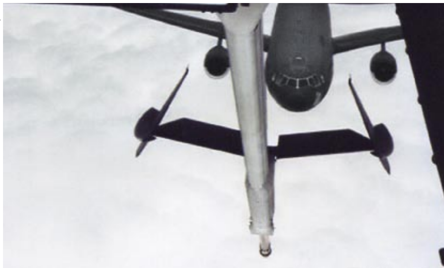
A KC-10 like Gold 11 prepares to take gas from the boom of another KC-10. This “give and pass” capability is unique in the tanker world.
