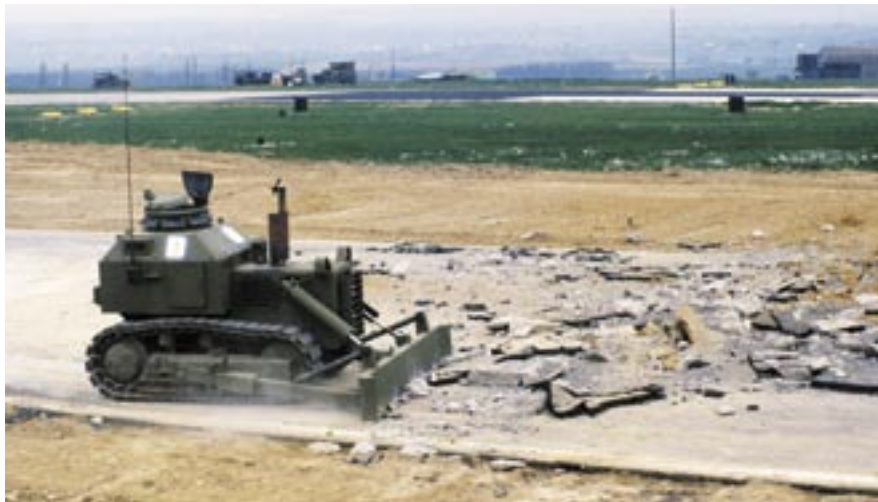
An armored bulldozer clears debris and live ordnance from the runway after one bombing run during the base survivability exercise.
