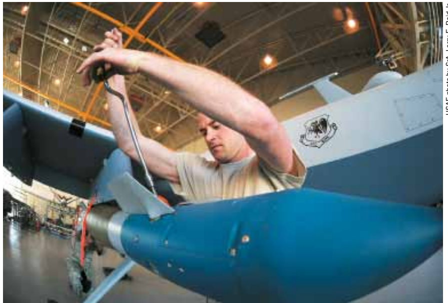
SrA. Jason Atwell secures the fins of a GBU-12 Paveway II laser guided bomb at Creech AFB, Nev. There is so much demand for Predator expertise that training is now also being done by the California ANG.
