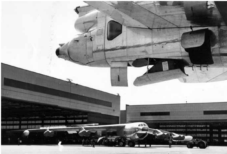
Above: A B-52F rolls out (back). In the foreground is a tail detail, showing, from left to right, the ammunition access door, the drag chute compartment, and the gunner's entry hatch. Right: Maintainers service the four .50-caliber M3 machine guns in the tail of a BUFF.
