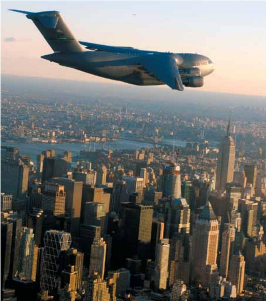
**A C-17 on the first transcontinental flight fueled by a synthetic fuel blended with JP-8 passes over New York City in 2007. The Air Force plans to certify its aircraft on other synthetic fuel blends as soon as possible.**
