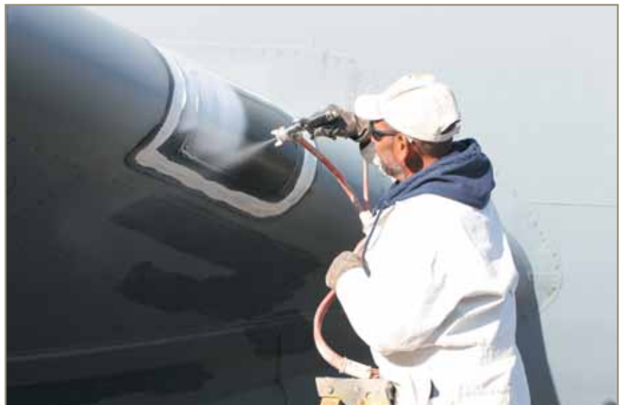
Top: It’s not just old airplanes. The tooling for the B-2 stealth bomber cockpit sits near retired bombers. A special treatment helps protect it from the elements. Above, Carlo Marinaz applies Spraylat to the forward edge of a KC-135’s wing.
