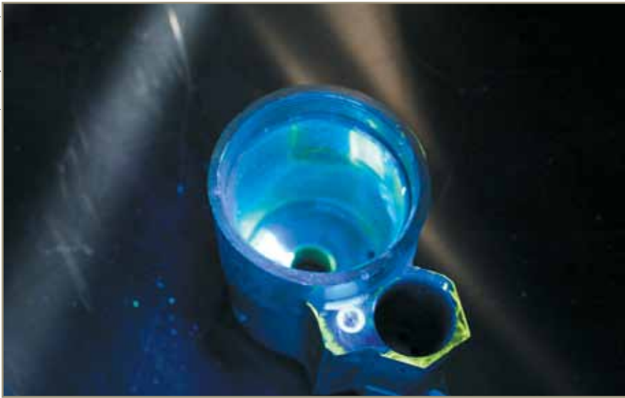
If asked, AMARG will test parts, looking for fatal flaws. Here, a part soaked in a fluorescent dye reveals cracks and other imperfections under black light.
