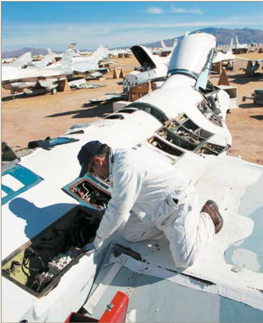
Left: Joe Gasak removes a flaperon bracket from an F-16. Hill AFB, Utah, urgently needed the part. It would probably get there within three days of the request. Above, another heavily harvested F-16 looks less like a fighter all the time.
