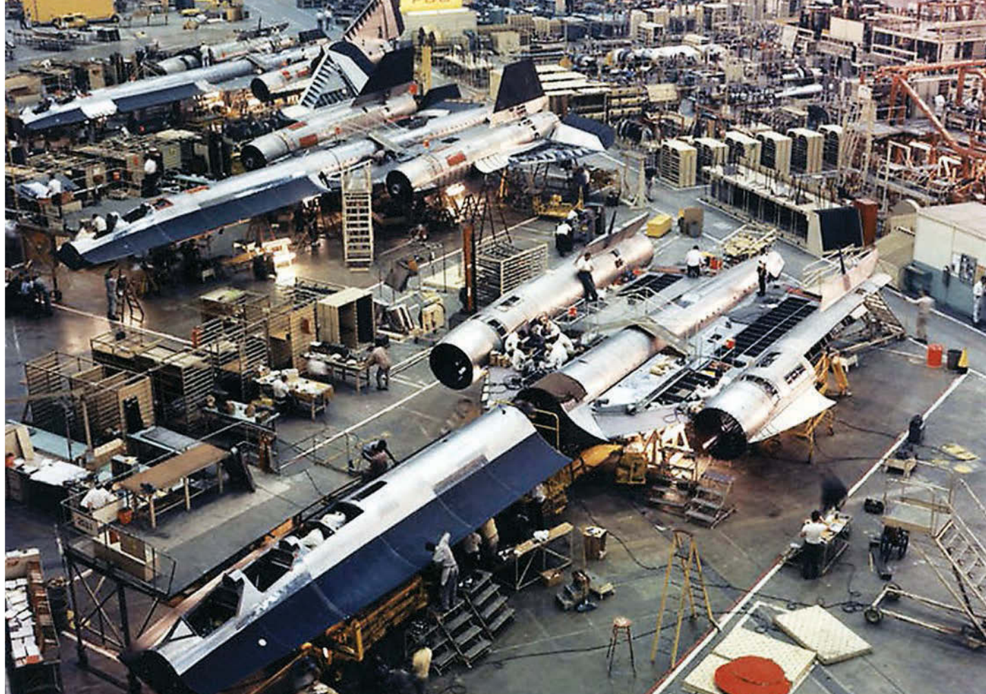
A-12s—secret CIA spyplanes that were forerunners of the SR-71—under construction when Skunk Works was located in Burbank, Calif.
