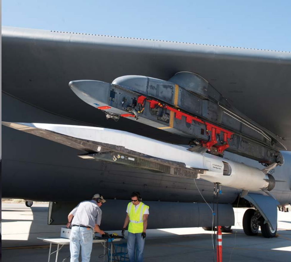
A ground crew makes the final checks on the X-51A Waverider scramjet before its second test flight in 2011. Former Air Force Chief Scientist Mark Lewis said the Waverider was a huge success that wasn't built on. Additional test flights could have yielded a great deal of hypersonics knowledge for little cost.
