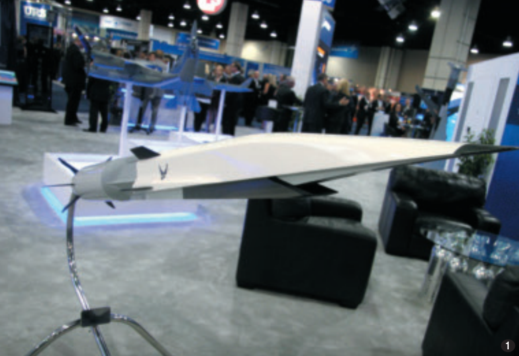
111 The pathfinder for the High-Speed Strike Weapon is the X-51 Waverider, shown off as a model by Boeing. The real X-51 achieved a flight of more than 300 seconds at speeds up to Mach 5 in May, providing a wealth of data for aerospace technologists to study. The project was a joint effort of DARPA, NASA, the Air Force, Boeing, and Pratt & Whitney. 121 Textron Chief Executive Officer Scott Donnelly speaks with Maj. Gen. Kenneth Merchant, director of USAF Global Reach Programs, in front of the Textron display. 131 Pratt & Whitney's large model display emphasized its key role in providing propulsion for USAF's top fighter aircraft (l-r): the F-15, F-16, F-35, and F-22 as well as the KC-46 tanker. 141 A C-130J propeller (background) made by Dowty and a Goodrich ACES 5 ejection seat with elements that can be retrofitted to the ACES 2, used by a large portion of the combat fleet, on display.
