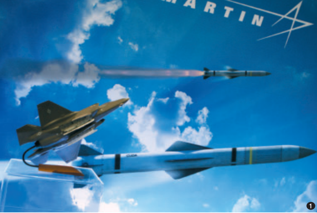
111 Lockheed Martin's Cuda missile is intended to increase the F-35's loadout without resorting to unstealthy carriage on the wings. A dozen of the radar guided hit-to-kill missiles could be carried internally on the F-35. Steering is aided by bursts from a belt of thruster ports. 121 Brig. Gen. Burke Wilson (r), director of space operations on the Air Staff, enjoys a moment with CMSgt. Rodney Reyes (l). 131 A Boeing satellite orbited above the company's booth. Boeing promoted its GPS IIF system as well as hosted payloads for government/commercial partnerships.
