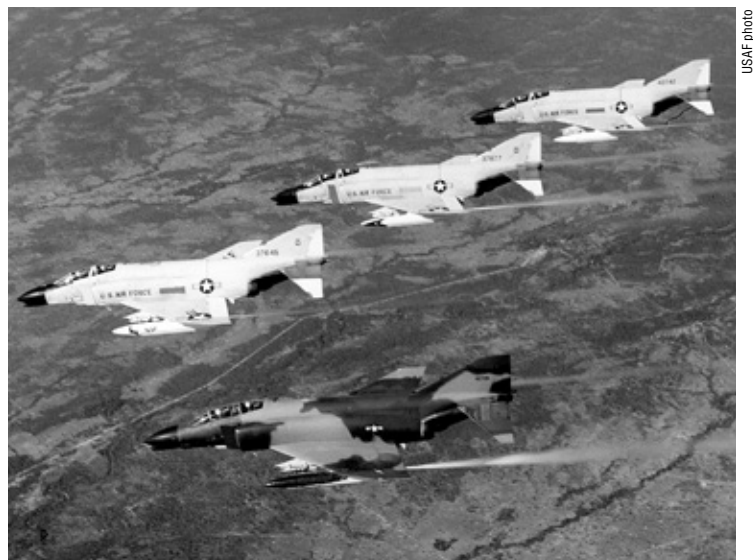
A four-ship formation of F-4 fighters. The early Phantoms were painted gray (see top three), but by the mid-1960s they were painted in a camouflage scheme (see bottom airplane).
