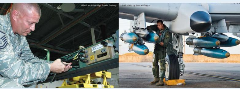
*MSgt. Brian Mosier adjusts an SDB II pneumatic carriage system used to mount the weapon on the aircraft.*
