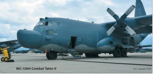
Iridium communications suite, troop/cargocapable cabin, casualty evacuation capability, NVG compatibility, and STOL austere operations enhancements. The aircraft first deployed in support of USAFRICOM operations in 2011. FY18 funds support navigation enhancements to permit ops in GPS-degraded environments.
