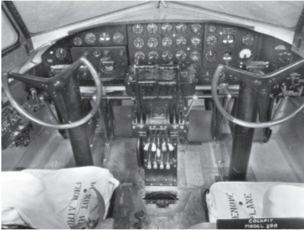
The cockpit of Model 299. The controls were not ergonomically designed. Right: Boeing's bombardment airplane in pieces at Wright Field, Ohio, in 1935. The crash killed two crew members and destroyed the airplane.
