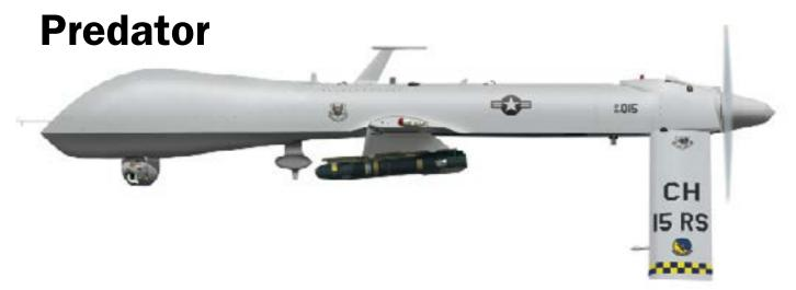
Predator, a remotely piloted aircraft, became world famous as the first successful weaponized RPA and first to conduct lethal strikes. Designed by General Atomics Aeronautical Systems, this medium-altitude, long-endurance system was first used by USAF for surveillance. Later it was armed with laser guided missiles and flown against terrorist targets. Many lethal missions were CIA ventures, but the aircraft, pilots, and command and control systems belonged to the Air Force.
