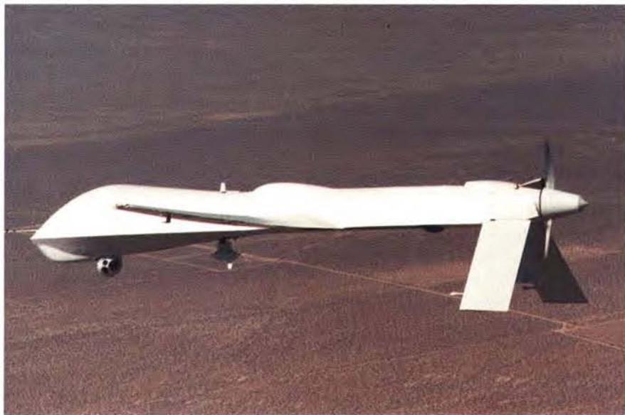
**Without displays, life-support gear, or other necessities of piloted aircraft, Predator UAVs and future UCAVs can be much smaller than fighters. They can also ignore human tolerances and achieve plus-or-minus twenty-G capability.**
