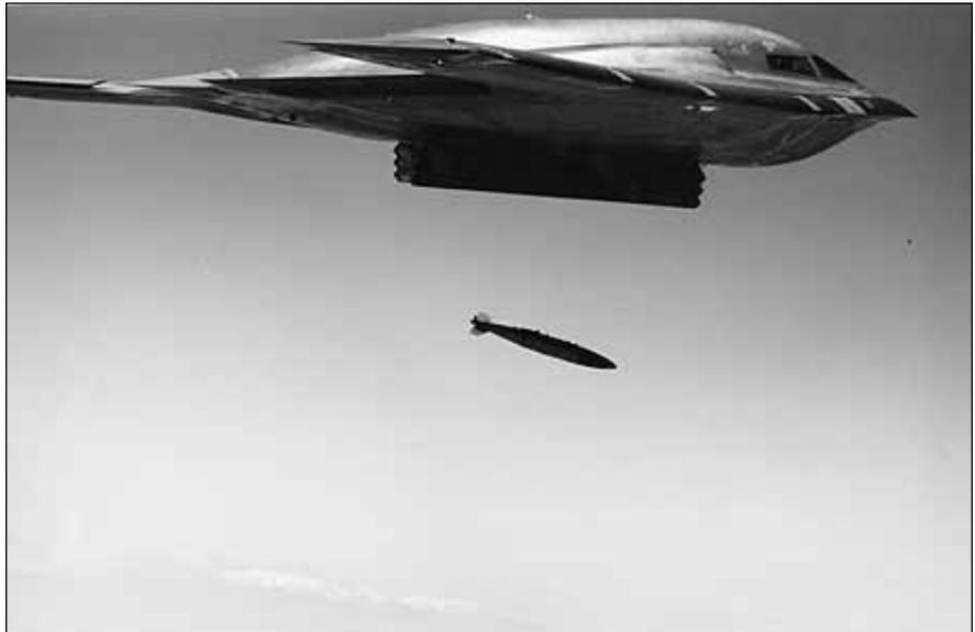
*At top, a B-2 takes on fuel from a KC-135 during an Operation Allied Force mission. Above, a Block 20 B-2 uses the GPS-Aided Targeting System to guide a munition during testing. In Allied Force, the combination of the Block 30 B-2's GATS with the JDAM produced outstanding accuracy.*
