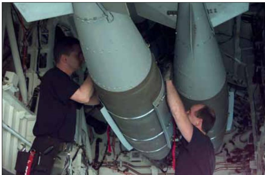
The other part of the B-2 success story was the Joint Direct Attack Munition, a 2,000-pound version of which is shown here being loaded in the B-2's bomb bay. Global Positioning System coordinates guide the JDAM to the target in any weather.
