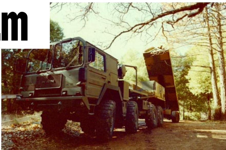
*The Ground Launched Cruise Missile, with its combined transport and launch vehicle shown here, had a short operational life but proved to be an effective counter to Soviet SS-20 intermediate-range missiles.*
