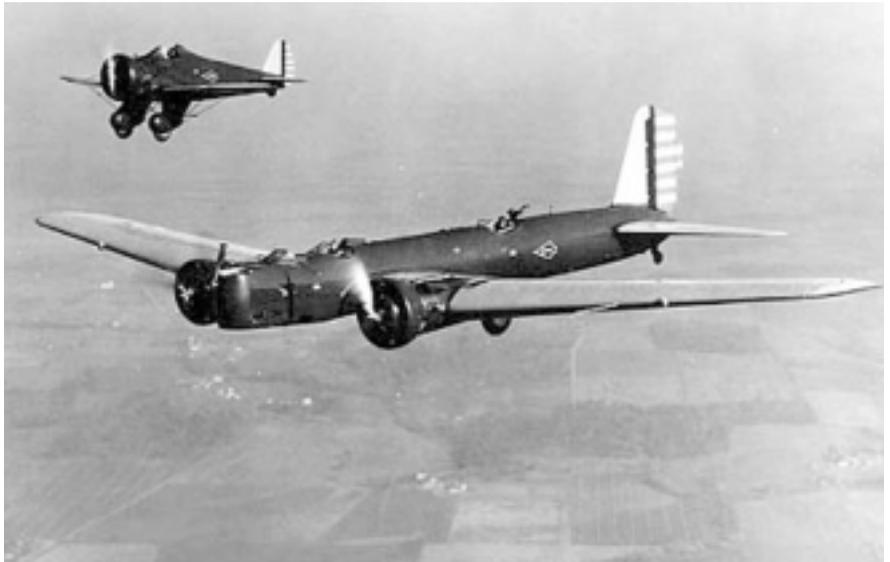
*The B-9 bomber (shown here with a P-26) was the first of several advanced aircraft introduced in the 1930s. The twin-engine, all-metal bomber featured retractable landing gear, cantilevered wings, and a top speed of 186 mph.*
