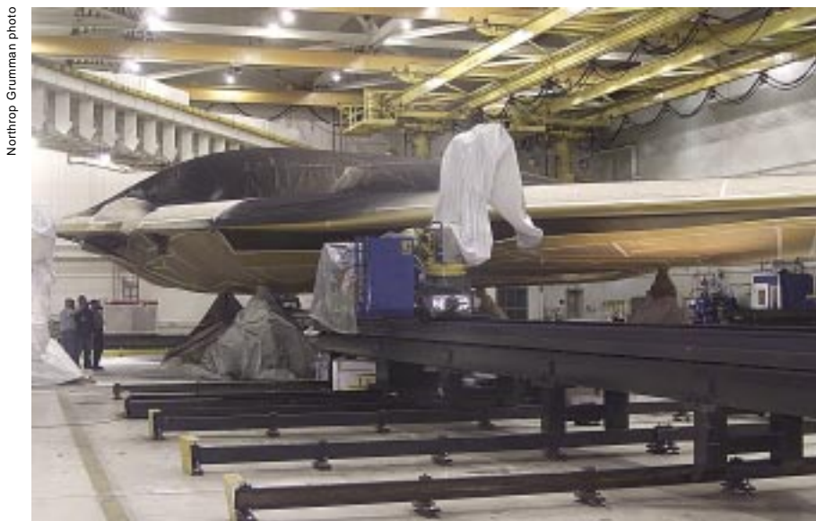
Upgrade. B-2s are getting a new stealth coating that will improve their combat readiness. USAF plans upgrades to each of its current bombers to keep them viable, even as it moves to field a new long-range strike system.
