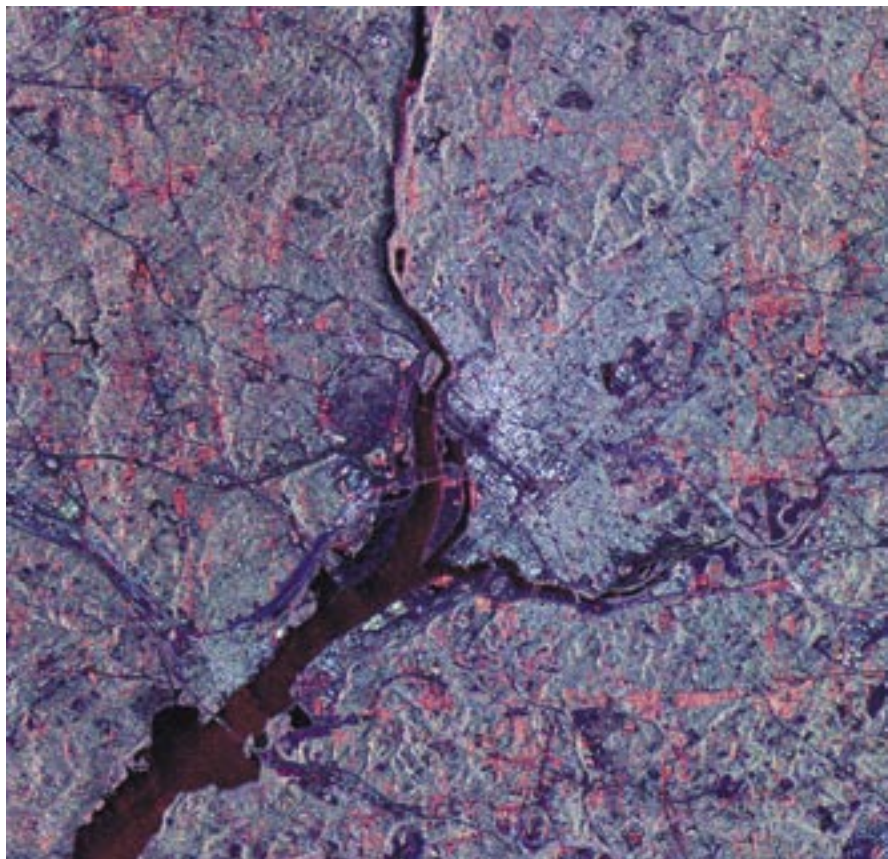
The Greater Washington, D.C., area shown in an image taken by a space radar. One of the benefits of space radar is that it can penetrate clouds.
