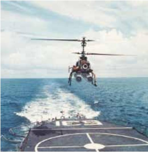
**A remotely operated DASH comes in for a landing on the deck of a US Navy destroyer. Plans called for DASH to deliver a nuclear depth charge.**
