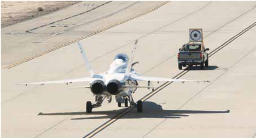
The F/A-18 research aircraft follows a pickup carrying an airborne tanker drogue image down a runway in early AARD testing. An RPA's approach to the boom is broadly based on optical recognition, aided by algorithms to improve prediction accuracy.
