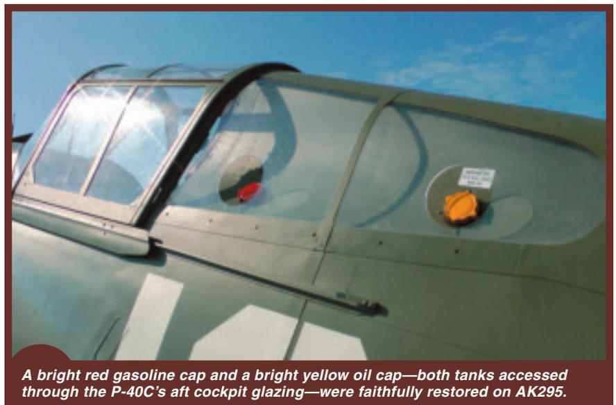
*A bright red gasoline cap and a bright yellow oil cap—both tanks accessed through the P-40C’s aft cockpit glazing—were faithfully restored on AK295.*
