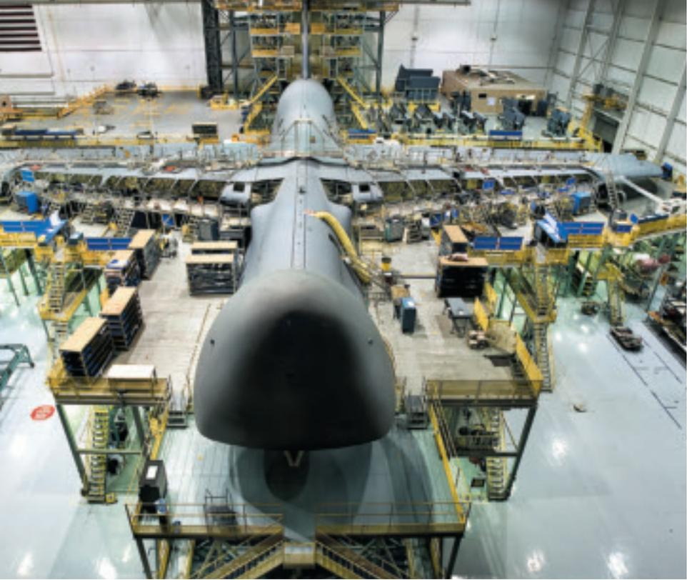
*Far left: SSgt. Jason Siverling adjusts a strap on a C-17 before a drop in South-west Asia. Left: A C-5 is transformed through re-engining and refurbishing into a C-5M Super Galaxy at a Lockheed Martin facility. Selva says the C-5M has "magnificent capability."*
