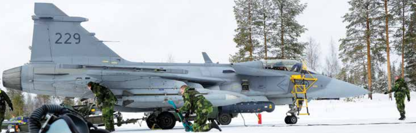
Swedish air force maintainers refuel and rearm a JAS-39 Gripen. The fighter is certified to carry many US munitions, and Sweden is seeking certification for more.
