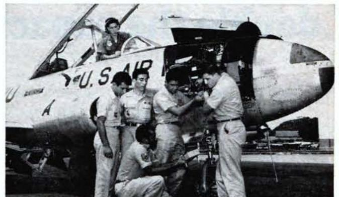
**Uruguayan Air Force personnel at USAF School for Latin America train as flight-line radio repairmen on both piston-engine and jet-aircraft radio systems. Here bilingual instructor demonstrates use of multimeter to check out T-33 communication system. After graduation, Uruguayans will become electronic specialists for units back home.**
