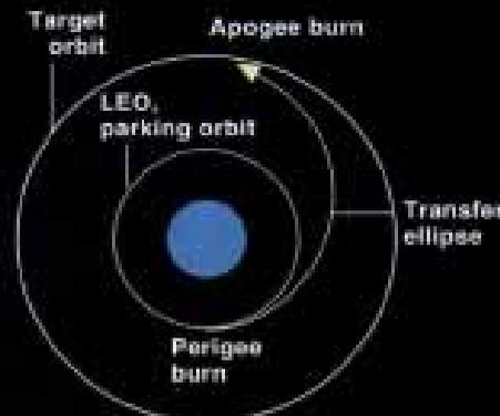
It is common procedure to pick an initial "parking" orbit, usually at LEO, then boost payloads to higher altitude. Engines are fired first (at perigee) to reach the apogee of an elliptical transfer orbit and then are fired again to put the spacecraft into a circular orbit at that higher altitude.
