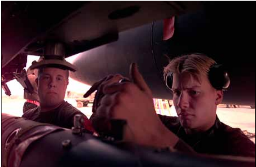
Deployed to Aviano AB for Operation Allied Force, 494th Fighter Squadron load crew members from RAF Lakenheath, UK, prepare to attach a GBU-24 laser-guided bomb to an F-15E.
