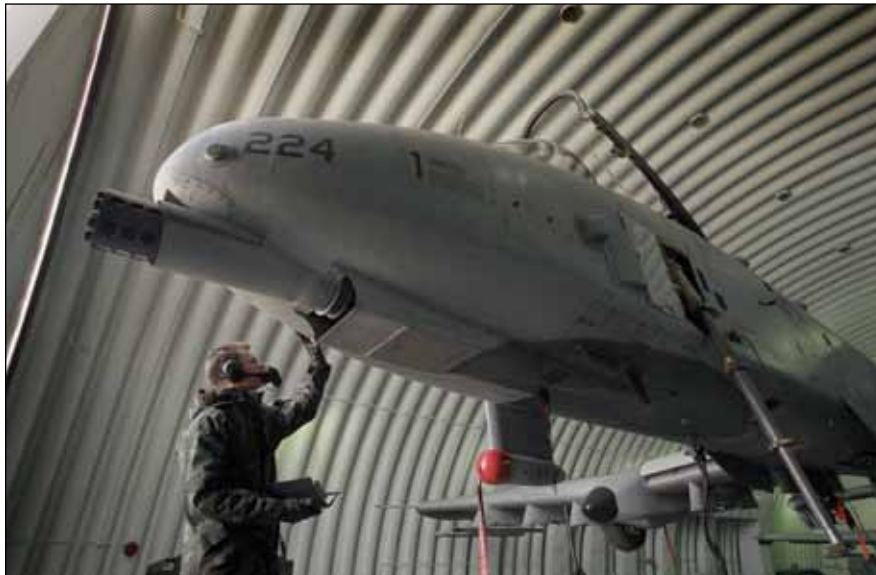
PACAF is a US forward presence that helps ensure stability in the Pacific Rim. Above, at Osan AB, South Korea, SrA. David Switzer inspects an OA-10 for proper panel fit during a landing gear retraction check.
