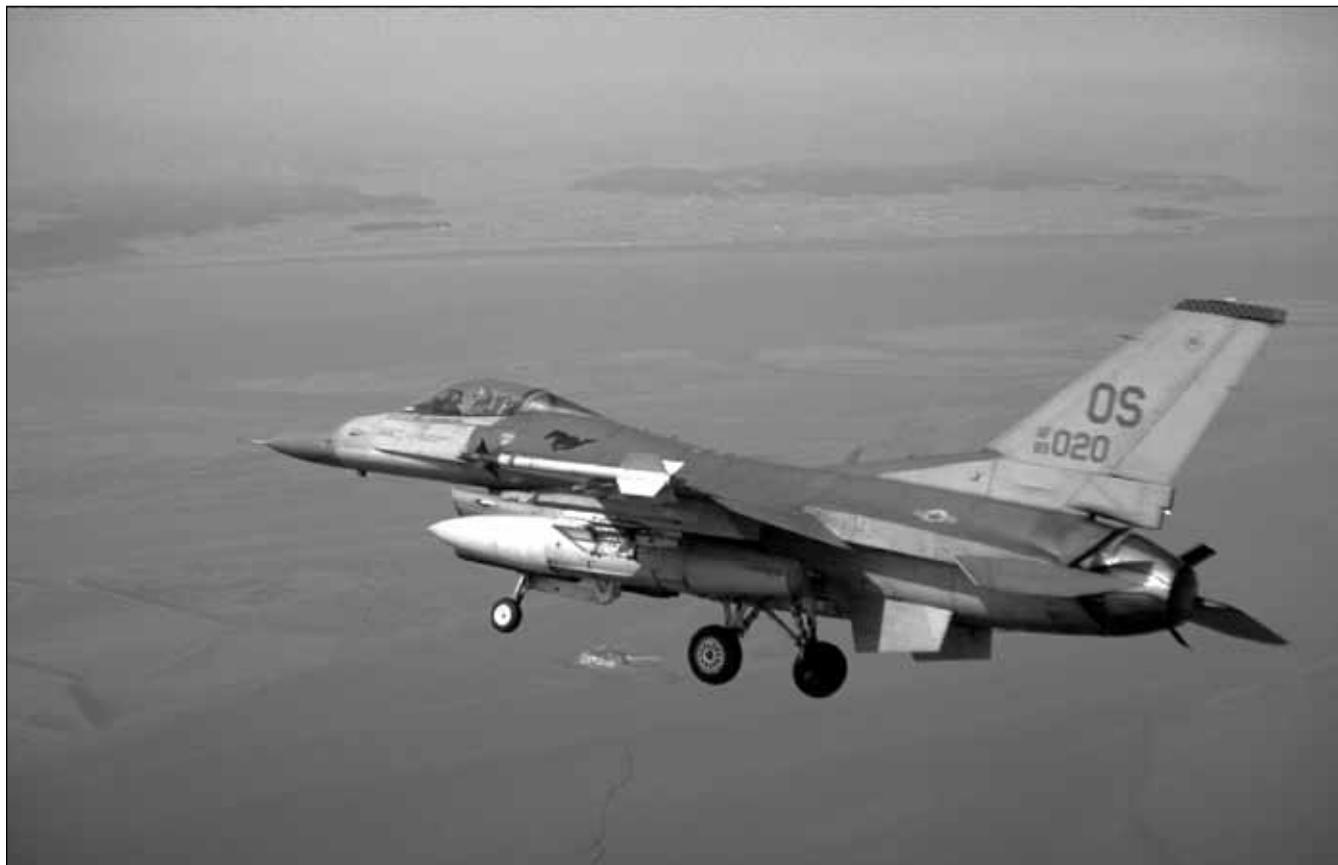
*The 36th FS—the “Flying Fiends”—operate the F-16CG, which is capable of carrying the Low-Altitude Navigation and Targeting Infrared for Night system. LANTIRN is a set of pods mounted under the F-16—one for seeing in the dark, the other for designating targets for laser-guided bombs.*
