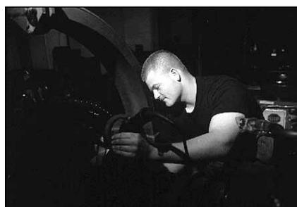
Responsible for more than 150 F-16 engines from the three air bases, squadron personnel take from 18 to 36 days to overhaul an engine, and on any given day they have about 20 in various stages of repair. These skilled and meticulous maintainers disassemble the engines, making upgrades or replacing parts, reassemble the engines, and test them in the hush house.
