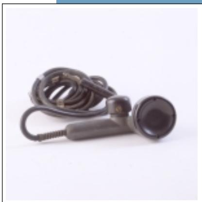
It is a T-17 carbon granule microphone with push-to-talk switch and five-foot-long rubberized cord. For Korean War veterans, though, it might evoke memories of calling in an airstrike or calling out an alert for MiGs or maybe even calling home via radio.
