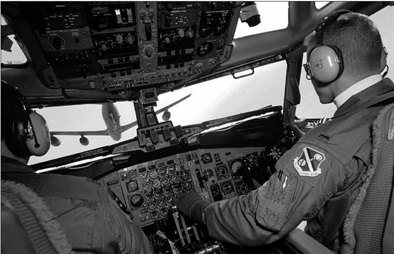
*On this mission, the flight crew takes on fuel from aircraft of the 19th Air Refueling Group, also based at Robins. Above, Lt. Rob Southerland carefully maneuvers the E-8C behind the tanker. The refueling receptacle is slightly behind the cockpit. Each pilot on the flight will conduct the refueling "dance."*
