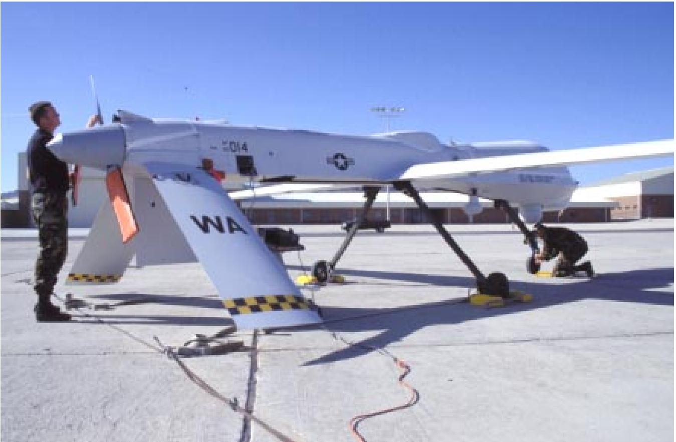
*The RQ-1 system can be broken apart into six main components and loaded into what the crews term "coffins" for rapid deployment worldwide. The GCS is the largest component, and it can be rolled onto a C-130.*
