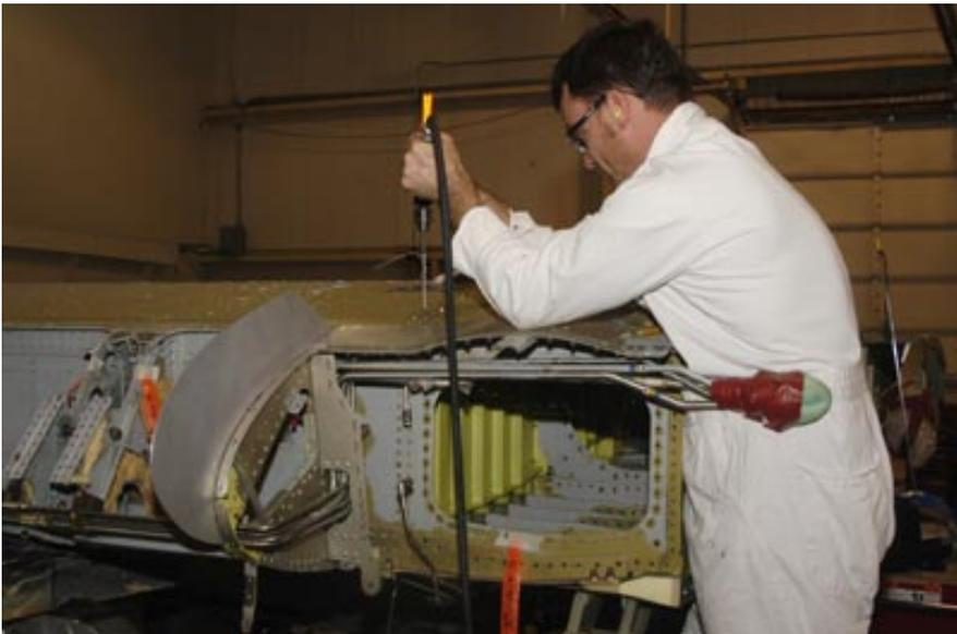
**The facility completed its first A-10 SLEP wings in 2003. At present, it takes about 140 days to complete a set. Each wing has its own individual quirks and problems; many of the repairs are “handmade” in nature.**
