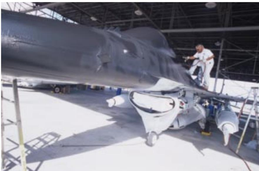
**At left, AMARC aircraft preservation technician Manny Vasquez applies a coat of Spraylat to an F-16. Aircraft arriving at the facility go first to this long open shelter. Workers drain all fluids and begin the process that will preserve the fighter. Storage is customized for three different types of use—a return to flying, spare parts, or eventual disposal. In all cases, the ejection seat system is deactivated and aircraft seams are taped over.**
