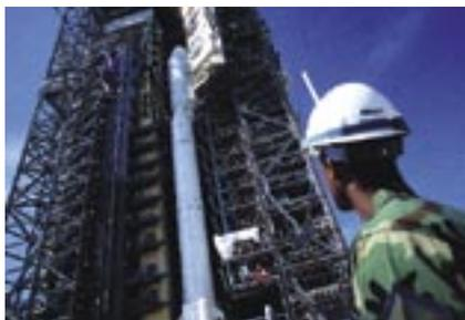
At top, the mobile service tower has been pulled back, leaving the launch vehicle in full view. Moving the million-pound tower without damaging the rocket requires extreme care. Above, MSgt. Lou Moyer, noncommissioned officer in charge of the 3rd SLS's booster section, observes as the door to the tower is prepared for rollback.
