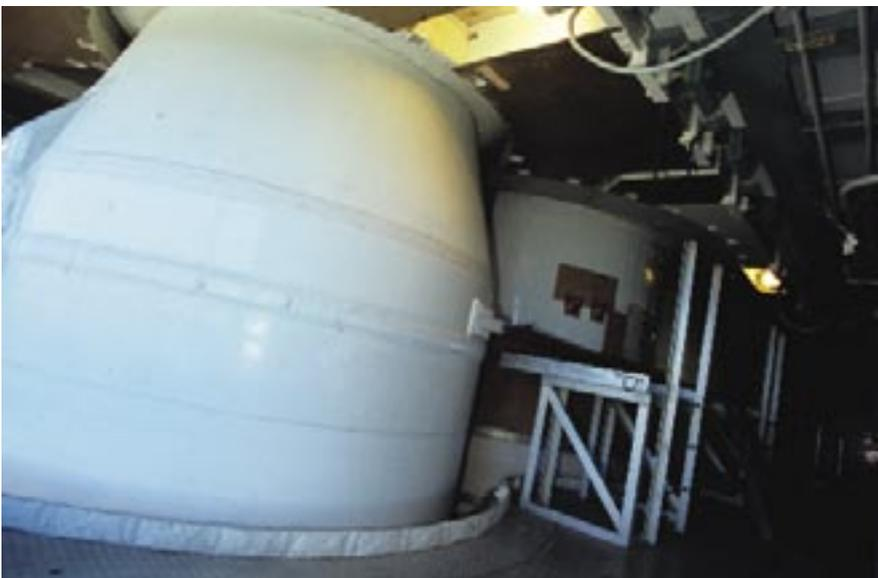
At left is the crucial joint where the Titan's solid rocket motors were mated to the main stages. The solid rocket motors fire first, lifting the rest of the launch vehicle.
