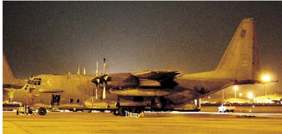
Top left, the AC-130's engines and external fuel tanks are clearly visible. Note the metal "bucket" covering the rear of the engine. These shrouds help block and suppress the heat signature of the aircraft's four turboprop engines.
