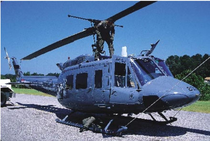
About all that's left from a UH-1H is the forward fuselage. The Huey II, undergoing a preflight inspection at left, has a longer, sleeker nose with space for avionics growth.
