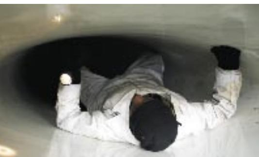
*The white-clad airman above is entering the air intake of an F-16 to check for engine blade damage.*
