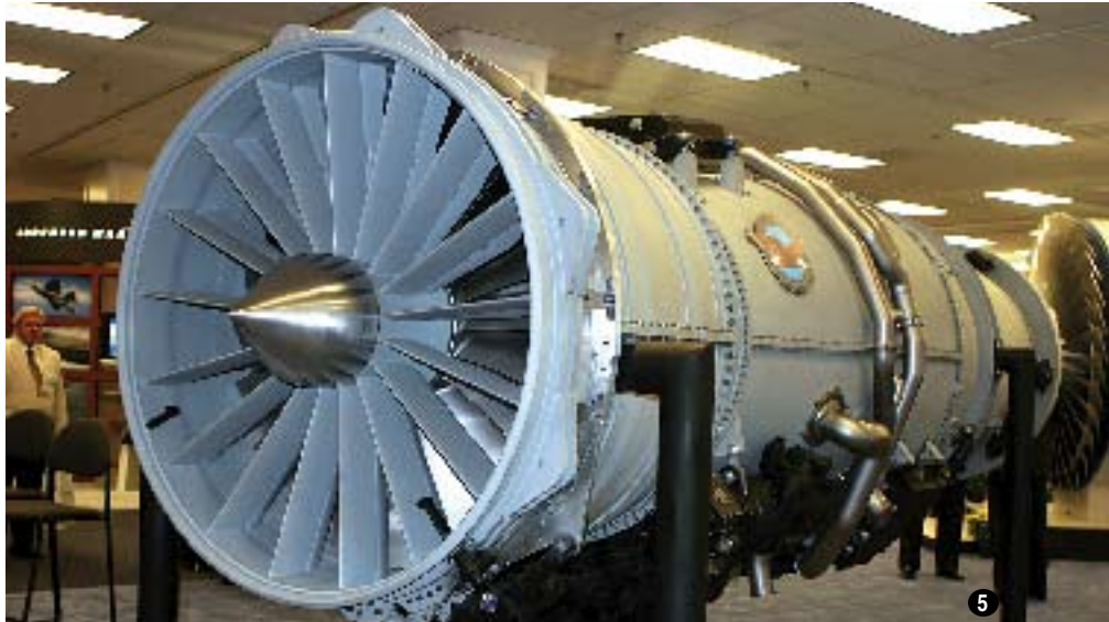
[5] A full-scale mock-up of the F135 engine that will power the F-35 fighter dominated the Pratt & Whitney booth. [6] Boeing displayed a cutaway of the
